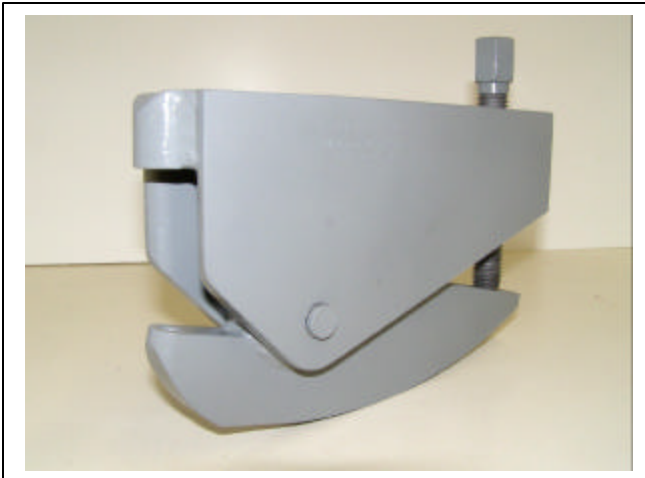
Door hinge pin press pictured above, steering wheel puller shown at right
